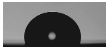
Figure 15. Contact angle measurement on a silicon wafer surface treated with an SAM of octadecanethiol.
